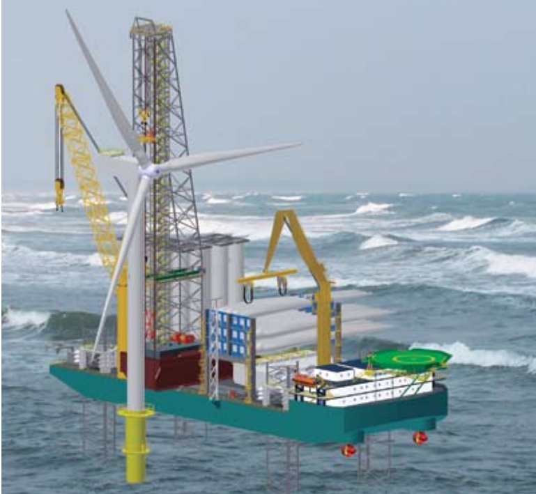
Image 1: A key feature of Keppel's OWI design is its ability to work in challenging weather conditions, especially in the presence of strong winds
