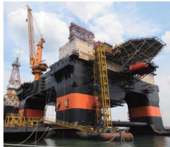
Keppel FELS was approached by Saipem S.p.A. to complete the commissioning of its Frigstad D90 semisubmersible rig, Scarabeo 9
