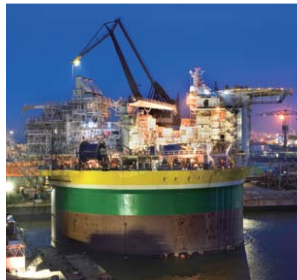
The world's first cylindrical FPSO facility, Sevan Piranema was completed by Keppel Verolme for Sevan Production in January 2007
